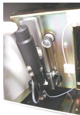
Photo 30 Push the piston down until the metallic clip will be over the aluminum hook then release the piston.
