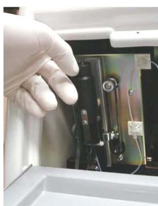
Photo 26 Pull firmly the piston assembly towards you so that the retaining magnets release the assembly.
