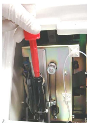
Photo 28 Replace the needle using the red or green tool tightening the new-one without excessive force to avoid damaging the plastic thread part.
