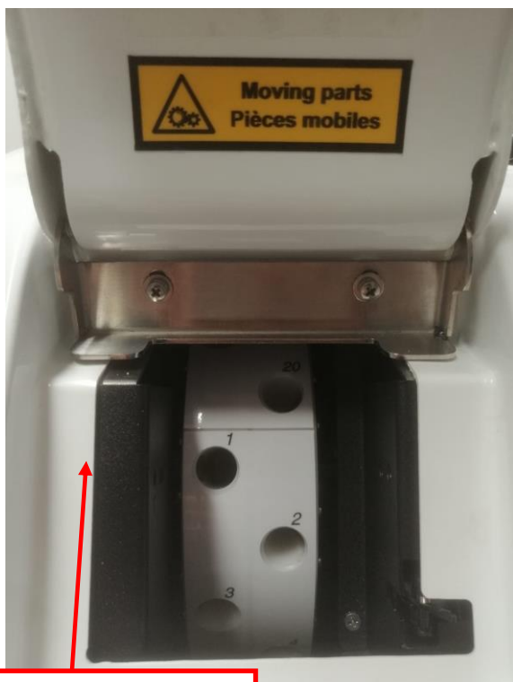
Inside detail of the Samples loading Door.
