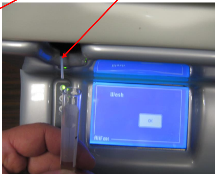
Retractable Tip for external withdraw (useful for tubes with plastic cap and/or paediatric tubes)
